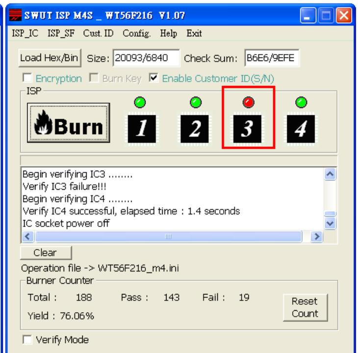
SWUT-M4S is 1-to-4 mass production programmer, and it also supports 1-to-1/1-to-2 or 1-to-3 programming. If no IC is placed in IC socket, no lights will appear on the corresponding IC ICON position while pressing “Burn” for programming and after programming is finished.
