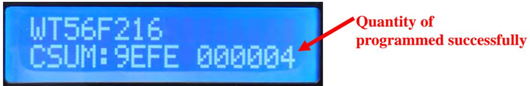
2. WT56F216 successfully programmed quantity has reached the limited quantity; 2 pieces of IC failed to programming correctly.
