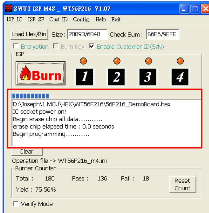
◆ After programming is completed, green light indicated successful programming; red lights indicated failure.
