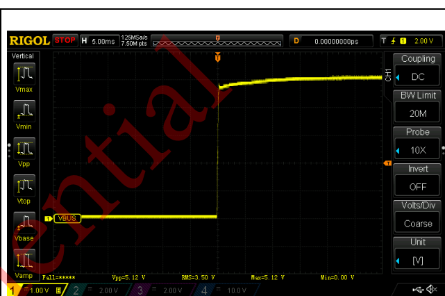
Figure 10 The start up waveform of Output at Vin = 90Vac/60Hz, 5V3A
