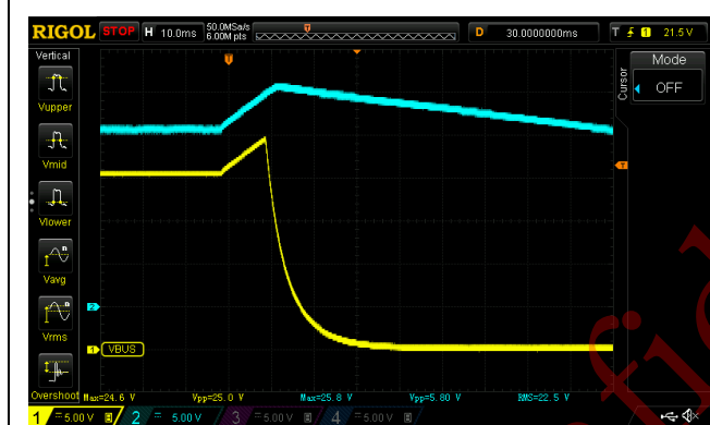
Figure 23 The waveform of OVP at Vin = 90Vac/60Hz, 20VNo-load
