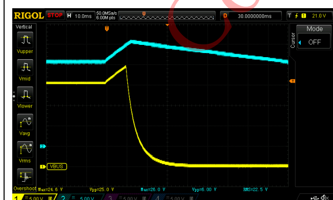
Figure 25 The waveform of OVP at Vin = 264Vac/50Hz, 20VNo-load
