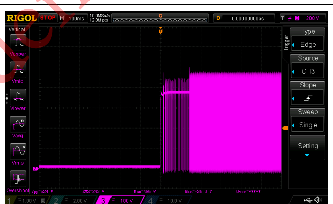
Figure 16 The waveform of Drain at Vin = 264Vac/50Hz, 5V3A Start up
